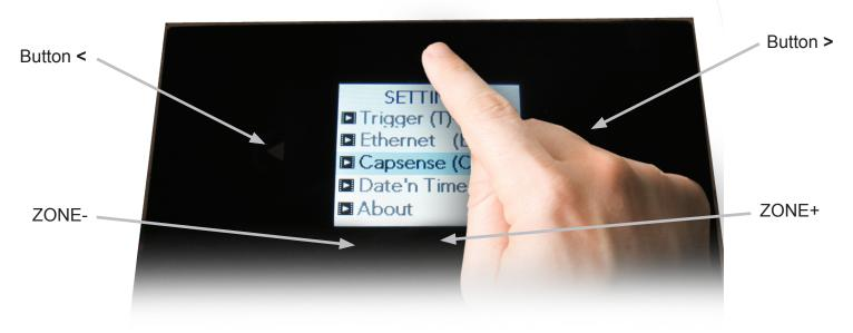
Press and hold the ON/OFF button for 3 seconds to get into the settings menu. Here are the available parameters:
